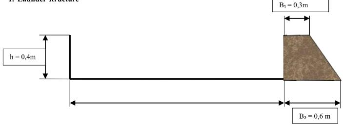
Slope is planned by the grader: h = 0,4m;  $B_1 = 0,3m$ ;  $B_2 = 0,6m$  on the whole length of road to be repaired.
